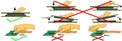
5. Precaution for soldering the LCM
